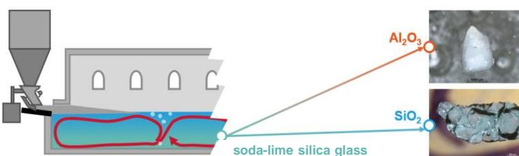
Preliminary studies on static dissolution have revealed that the kinetics of alumina dissolution in the glass melt during fusion are mainly controlled by diffusion at temperatures above 1400°C. However, these results have also shown that diffusion is coupled (oxides influence each other). In particular, alkaline-earth elements appear to play a special role. Industrial soda-lime matrices exhibit variability for these elements.
