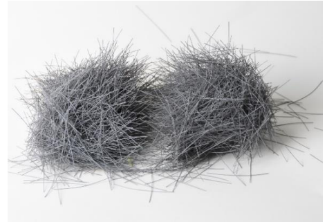
Figure 1 : Fracture of an aggregate of entangled model fibers.
