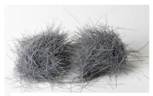
Figure 1: Break-up of an aggregate made of model entangled fibers.
